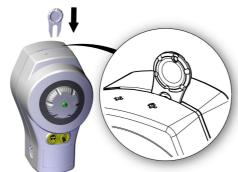
Insert the quick-prime key, on the right hand side of the slot
