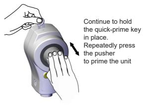
Once the unit is fully primed, remove the quick-prime key and press the pusher until you hear a click. The unit is now ready to operate normally at its original dose position
