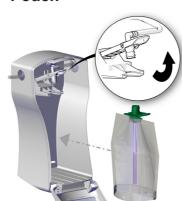
Lift the pouch lever and insert the chemical pouch
